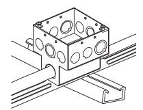
Secure to Unistrut with bolt and strut nut
