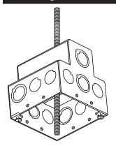
Secure to threaded rod with nut on top and below in the box
