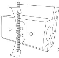
Depress the batwing clip until it securely clips onto ceiling wire or threaded rod
