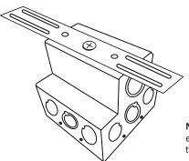
Secure to box hanger with 2x screws
